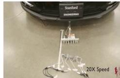
Now heavy objects need not be dragged into difficult areas by huge machines. This can be accomplished with these tiny robot ants! By using two simple wheels and controllable adhesives to apply interaction forces, these tiny robots are able to pull object more than their body weight! Get technical insights on these robots in this research paper from the library's subscription!
